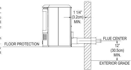
Figure 36 Minimum Exterior Grade Dimension - Unit Without Pedestal
